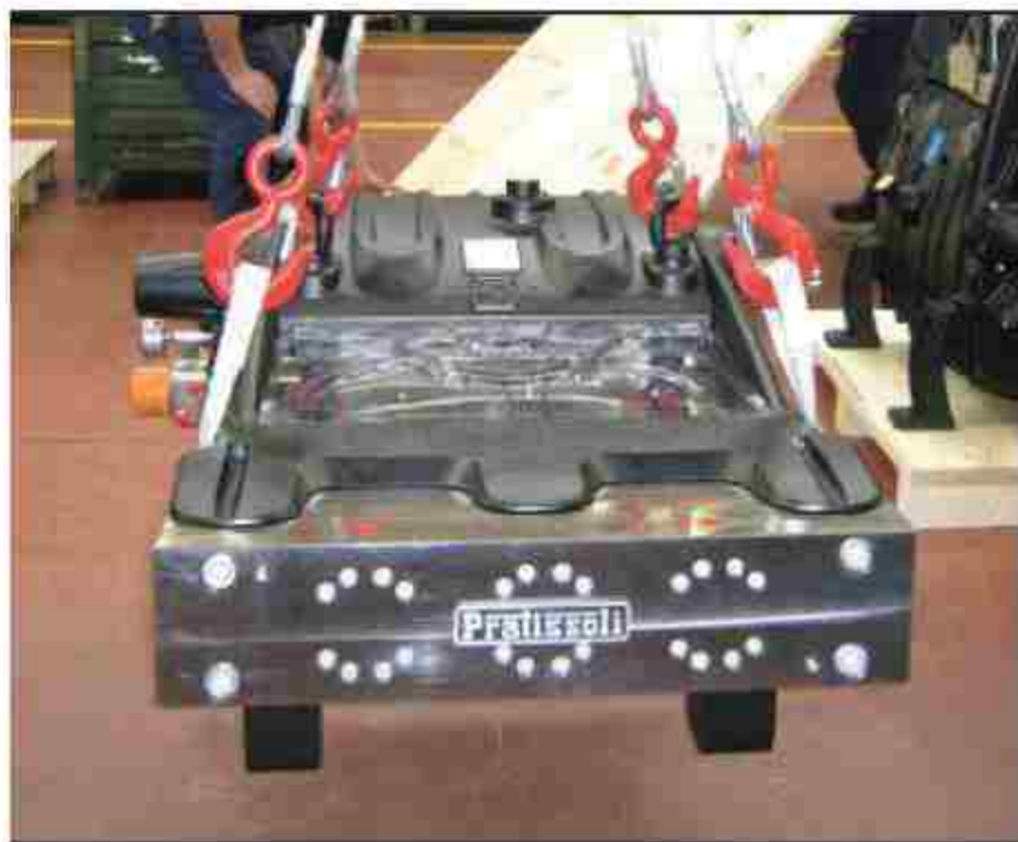
Standard Ultra-High Pressure made from Super Duplex SAF 2507
